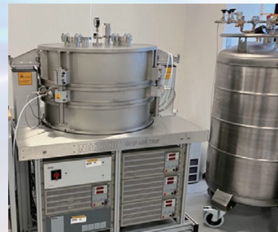
Cryogenic thermal conductivity measuring device
