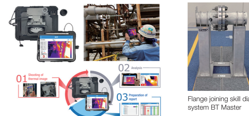
Energy-saving diagnosis system (an example of Thermofit)
