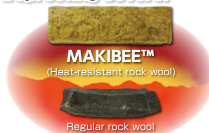
A shrinkage comparison of MAKIBEE and regular rock wool when left at 800°C.
