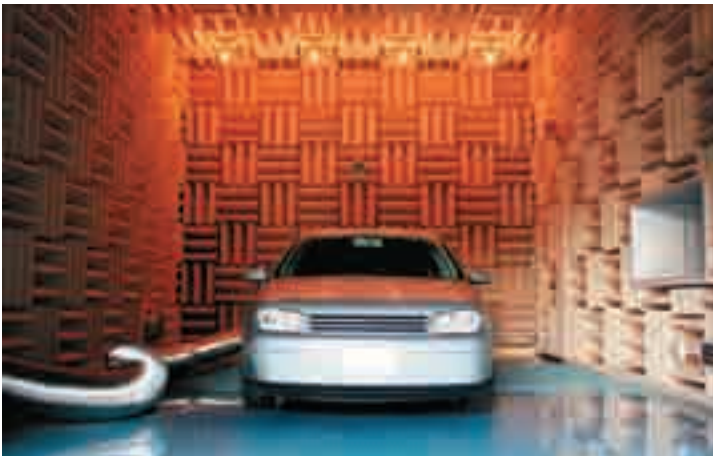
実車半無響室 Semi-anechoic chamber with an actual vehicle
