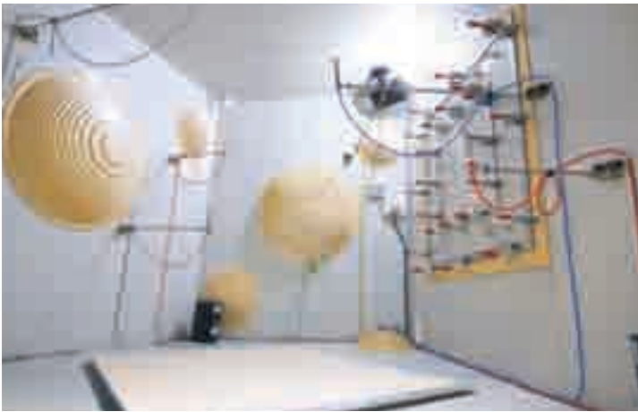
残響室法吸音率・音響透過損失測定システム Sound absorption coefficient and sound transmission loss measurement system (Reverberation chamber)
