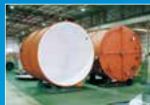
Fluoropolymer chemical tank lining
